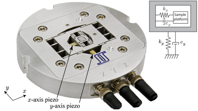
Fig. 4. Custom-made three-axis serial-kinematic piezo-based nanopositioner.
